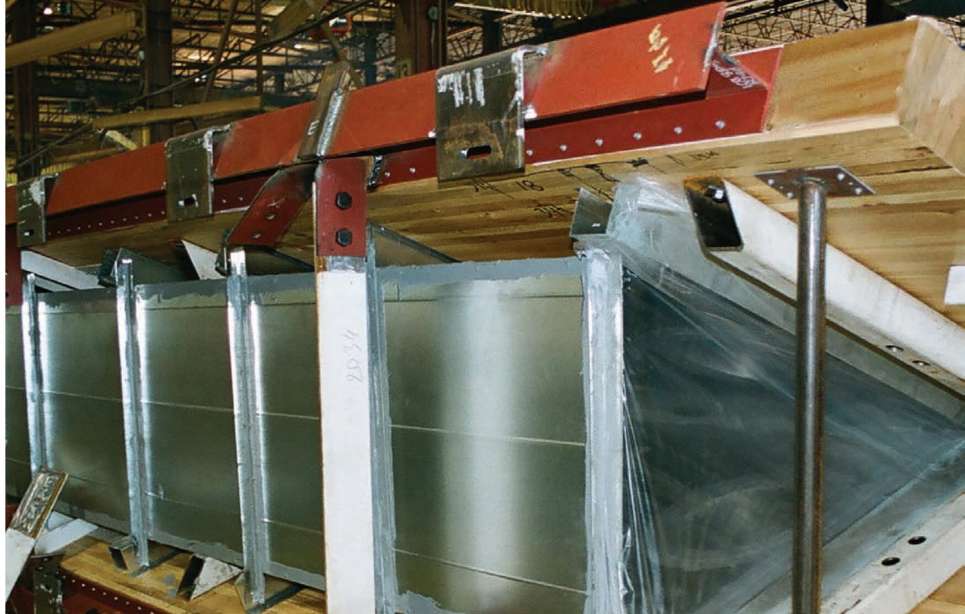
Glulam Arch section - fabrication details
